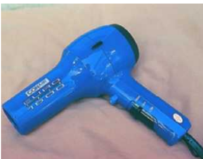
Figure 3.36 The number, 1600, indicates the maximum electric power this hair dryer may safely draw from the circuit.
