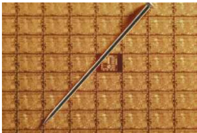
Figure 7.18 Enlarged image of a micro-electronic circuit etched on a semiconductor chip. The pin lying on top of the chip provides an idea of the extremely small scale of the circuit.
