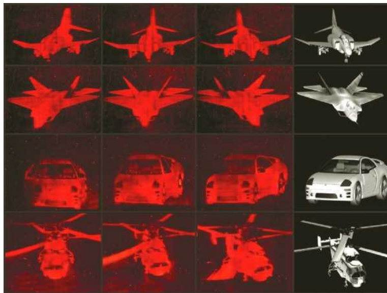
Figure 10.45 Holograms of four different vehicles (shown in the far right panel) made using a diode laser. The holographic images to the left of each vehicle reveal their three-dimensional character insofar as different aspects of the vehicles are displayed depending on the viewer’s perspective on the scene.
