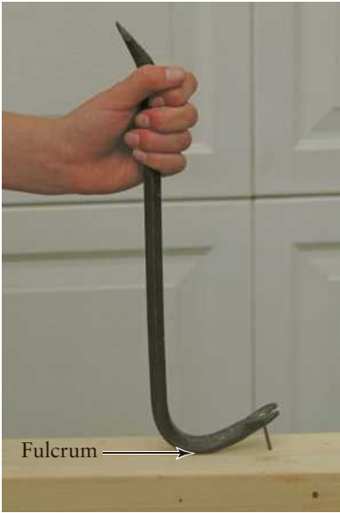
Figure 3.11 In using a crowbar to remove a nail from a piece of wood, a person does the same amount of work to complete the task as would be done in pulling it out using, say, a pair of pliers, but with a much smaller applied force.
