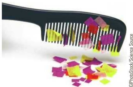
Figure 7.1 The amber effect. The comb attracts bits of paper because it was charged by rubbing.
