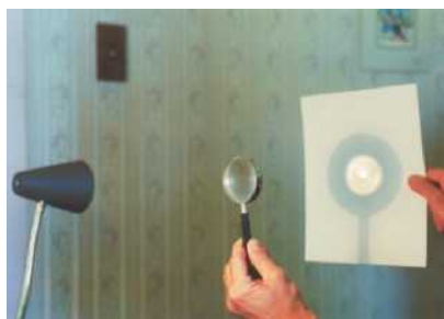
Figure 9.47 Single-lens image formation.
