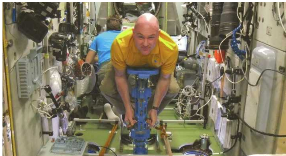
Figure 2.26 European Space Agency astronaut Andre Kuipers uses an inertial balance to measure his body mass in the Zvezda Service Module of the International Space Station.
