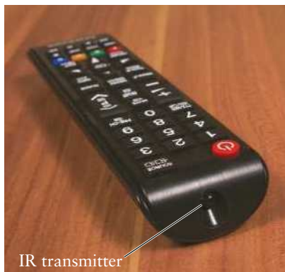
Figure 8.33 This remote-control unit uses infrared radiation to transmit signals to other electronic devices to control their operation.
