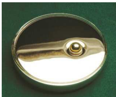
Figure 4.38 A steel ball floats in mercury because the density of mercury is greater than that of steel.
