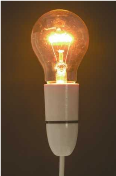
Figure 7.29 The current causes the thin filament wire to become white hot, even as the larger wires connected to it stay much cooler.
