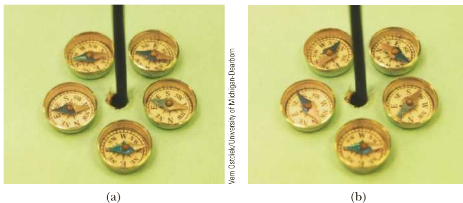
Figure 8.9 (a) The compass needles align with Earth's magnetic field when no current is in the wire. (b) The compass needles show the circular shape of the magnetic field produced by a large current (15 amperes) flowing in the wire.
