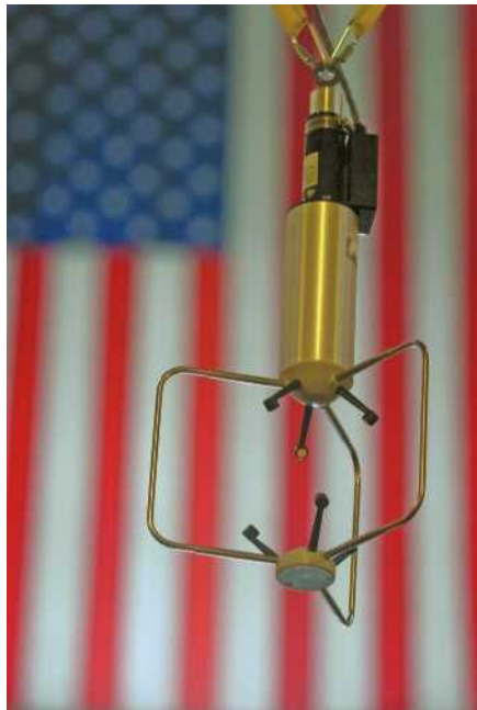
Figure 6.34 A sonic anemometer suspended in Grand Central Terminal in New York City is among the instruments deployed by the U.S. Department of Homeland Security to study the movement of air in the event of an emergency. Three ultrasonic transducers located at the corners of the two triangular devices serve as transmitters and detectors of sound pulses sent between them. Analysis of the pulse travel times between the various pairs of transducers can be used to establish the air speed and direction in the vicinity of the anemometer.
