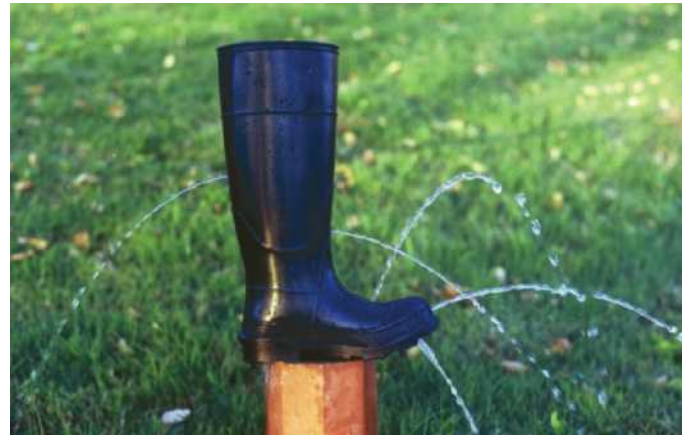
Figure 4.25 A rubber boot is filled with water. The pressure of the water acts on all parts of the inner surface of the boot and forces water out of any hole punched in the boot. The speed of the water coming out of a hole depends on how far the hole is below the surface of the water.
