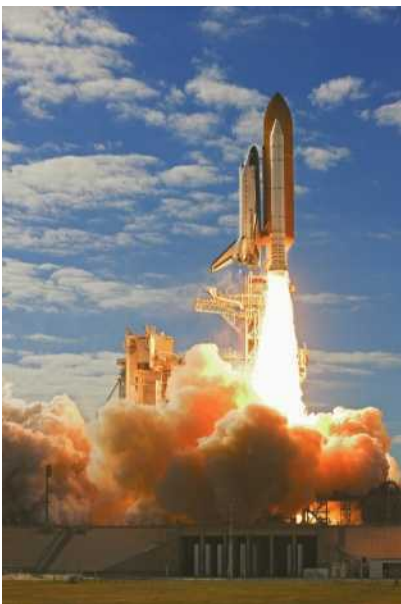
Figure 3.9 As rocket engines give momentum to exhaust gases, they gain momentum in return in the opposite direction.
