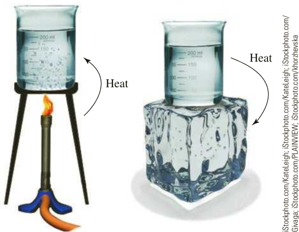
Figure 5.18 Heat flows into the water from the burner, increasing the water's internal energy. Heat flows out of the water into the ice, lowering the water's internal energy.
