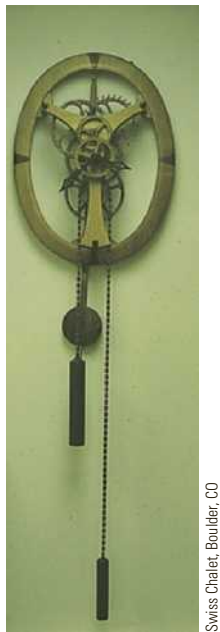
Figure 3.20 The source of energy to run this clock is the potential energy of the weights.
