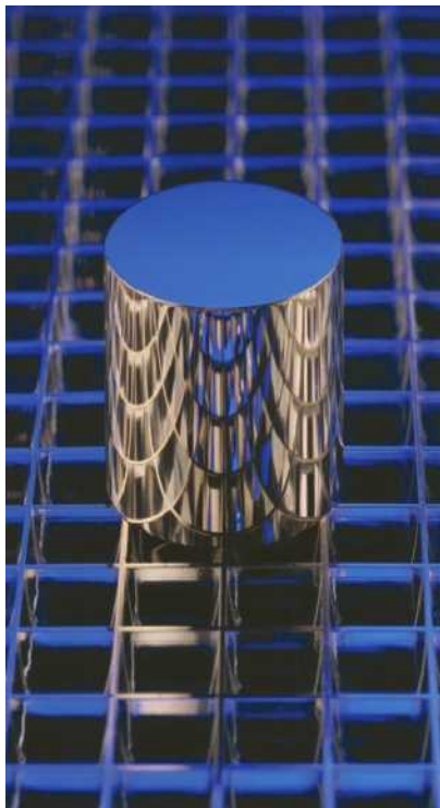
Figure P.6 The international 1-kilogram standard of mass, a platinum-iridium cylinder. This physical artifact will soon be replaced as the mass standard with a definition based on the fundamental unit of time, the second, and some agreed-upon fixed constants of Nature.
