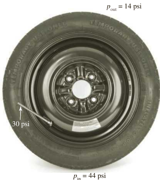
Figure 4.19 An absolute pressure inside of 44 psi produces a gauge pressure of 30 psi.
