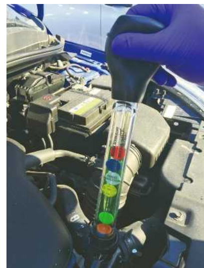
Figure 4.23 The freezing point of a car's coolant can be determined by measuring the coolant's density. This indicates the relative amount of antifreeze in the mixture. (See Section 4.5 for more.)
