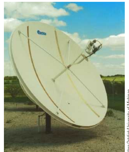
Figure 6.16 Parabolic dish antennas focus radio waves by reflection.
