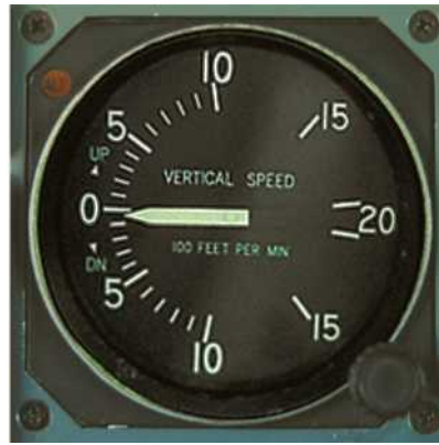
Figure 4.33 An altimeter (left) measures altitude by measuring the air pressure. A vertical airspeed indicator (right) measures vertical speed by measuring how rapidly the air pressure is increasing or decreasing.
