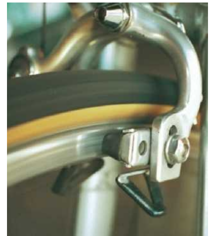
Figure 2.6 Bicycle brakes use kinetic friction as the pads rub against the rim of the wheel.
