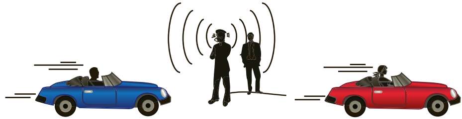
Figure 6.19 The Doppler effect with moving observers. The person in the car on the left hears a higher frequency than the pedestrian. The person in the car on the right hears a lower frequency.
